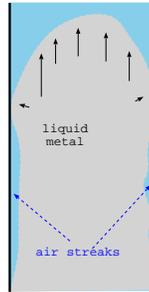
Fig. -3.6. Entrance of liquid metal to the runner.
