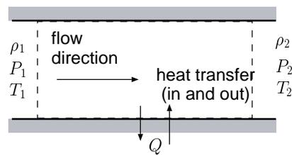
Fig. -11.1. The control volume of Rayleigh Flow.
