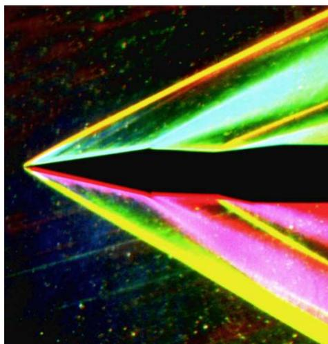
Fig. -14.11. Color-schlieren image of a two dimensional flow over a wedge. The total deflection angle (two sides) is  $20^\circ$  and upper and lower Mach angle are  $\sim 28^\circ$  and  $\sim 30^\circ$ , respectively. The image show the end-effects as it has thick (not sharp transition) compare to shock over a cone. The image was taken by Dr. Gary Settles at Gas Dynamics laboratory, Penn State University.
