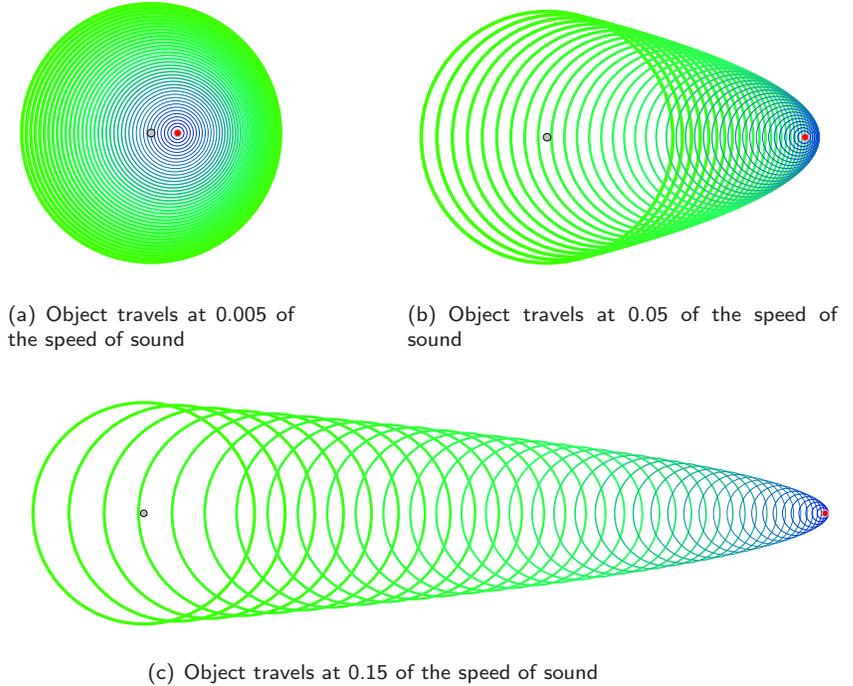
*Fig. -4.5. Moving object at three relative velocities. The gray point in the first circle is the initial point the object. The final point is marked by red circled with gray filled. Notice that the circle line thickness is increase with the time i.e the more green wider circle line thickness. The transition from the blue fresher lines to the green older lines is properly marked.*
