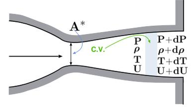
Fig. -5.4. Control volume inside a converging-diverging nozzle.
