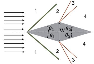
Fig. -15.7. A simplified diamond shape to illustrate the supersonic d'Alembert's Paradox.
