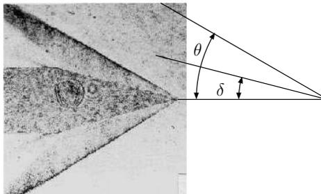
Fig. -14.17. Oblique shock occurs around a cone. This photo is courtesy of Dr. Grigory Toker, a Research Professor at Cuernavaco University of Mexico. According to his measurement, the cone half angle is  $15^\circ$  and the Mach number is 2.2.
