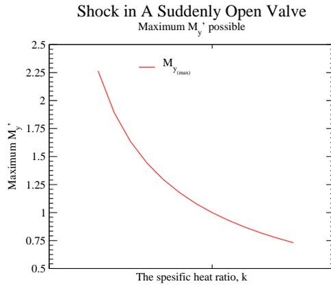
Fig. -6.15. The maximum of "downstream" Mach number as a function of the specific heat,  $k$ .
