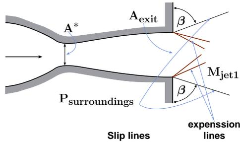
Fig. -15.11. Schematic of the nozzle and Prandtl–Meyer expansion.
