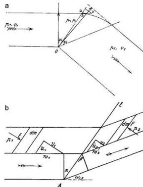
Fig. -1.13. The diagram is taken from Meyer's dissertation showing the schematic of oblique shock and the schematic of Prandtl–Meyer fan.
