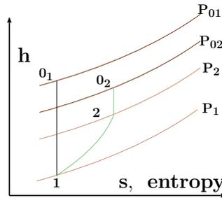
Fig. -7.3. Description to clarify the definition of diffuser efficiency.
