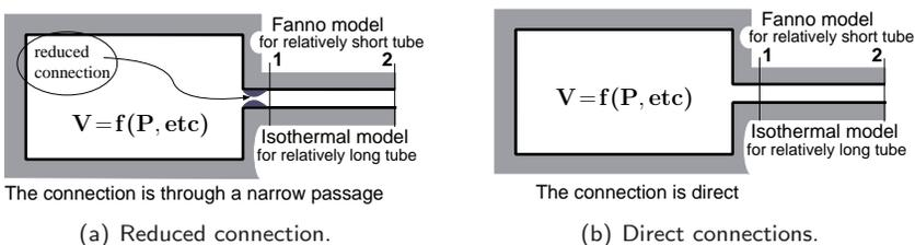
Fig. -12.2. Comparison direct and reduced connection. These two connection are two limits of the possible connections.
